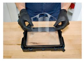
Put on gloves and align the SmartFilm, making sure the small notch lines up with the pour spout for proper orientation.
