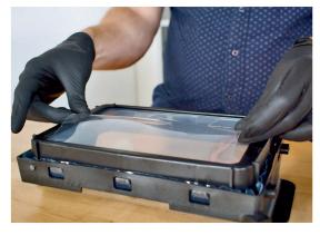
Insert rear tabs UNDER the frame, keeping SmartFilm centered and even.
