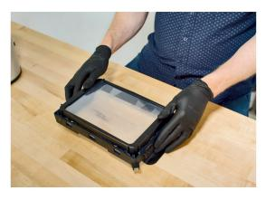
Press down around the edges to make sure SmartFilm sits flat and fully secured.
