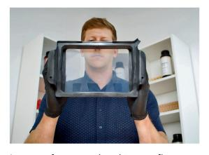
Inspect from eye level to confirm SmartFilm is flush.
